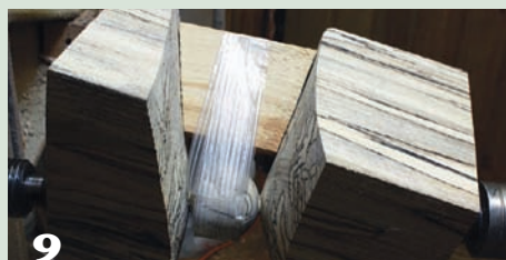
For security, strapping tape gives additional support for the wedge while turning.
