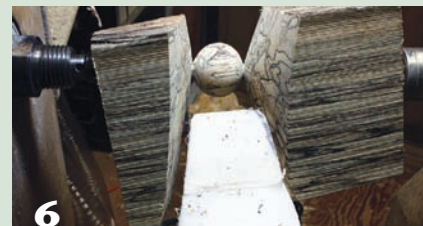
The toolrest is made from UHMW polyethylene.
