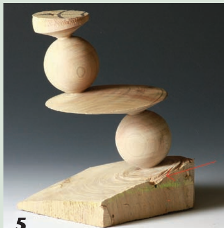
The tool tends to bounce when entering the wood after lingering in the “air wood,” especially when the speed is slow.
