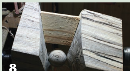
A wedge of wood hot glued into the V space supports the second axis.
