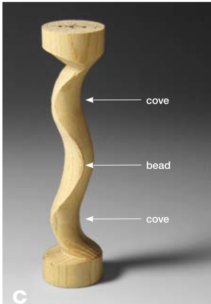
C An arc type spindle with two parallel axes shows the cove, bead, and cove .
