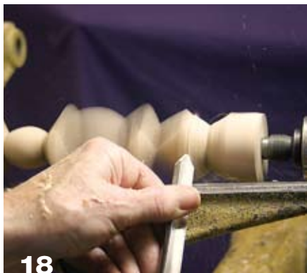
18 Return to Axis 1 (your fourth position) to make a V-cut at the tailstock end.
