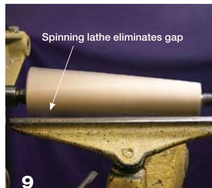
When the lathe is turning, the gap between the tool rest and air wood disappears.
