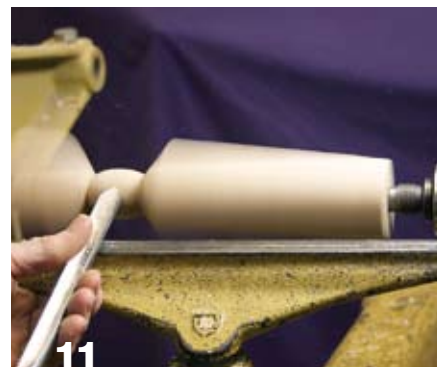
Position the tool tip high on the wood, which will allow the bevel to contact the wood.
