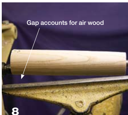
After mounting the spindle for Axis 1, adjust the tool-rest position (gap at left).
