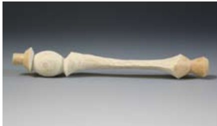
Here's one variation: The bottom bead, left , is a circular type and the right profile is an arc shape that is twisted.
